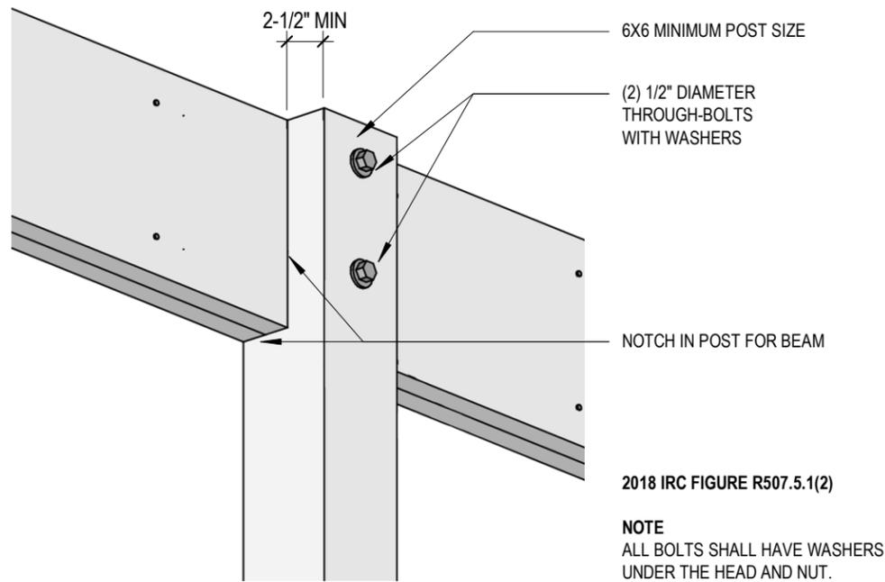
**3 ALTERNATE BEAM TO POST CONNECTION**
